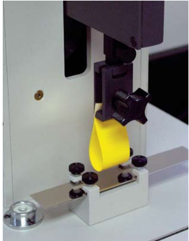
Figure 5. Loop fixture mounted in loop tack tester.
