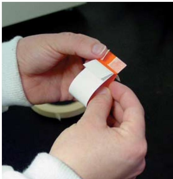
Figure 6. Creating loop specimen.
