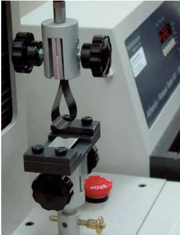
Figure 4. Tensile fixture mounted in tensile tester.
